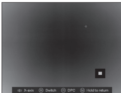
FIGURE 2-7. DEFECTIVE PIXELS CORRECTION
