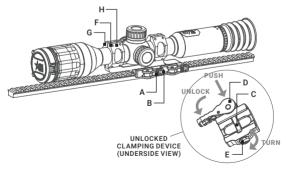
FIGURE 2-6. INSTALLATION WITH QUICK RELEASE MOUNT
