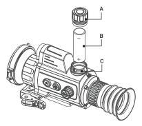
FIGURE 2-1. BATTERY INSTALLATION
