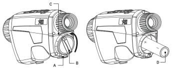
FIGURE 2-1. BATTERY INSTALLATION
