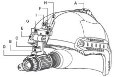
FIGURE 2-3. MOUNTING THE NVM TO A HELMET
