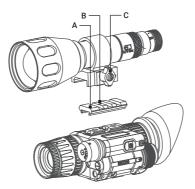
FIGURE 2-8. MOUNTING AN IR ILLUMINATOR
