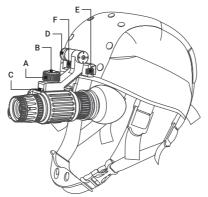
FIGURE 2-2. MOUNTING NVM TO A GOGGLE KIT
