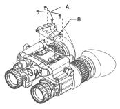
FIGURE 2-4. INSTALLING A MOUNTING BRACKET
