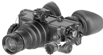
FIGURE 2-5. INSTALLATION OF THE IR SPOT/FLOOD LENS
