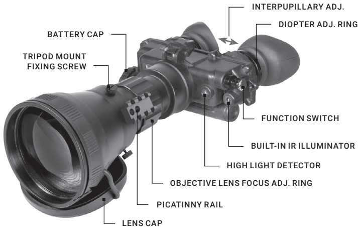
FIGURE 1-2. FOXBAT-LE MAIN PARTS
