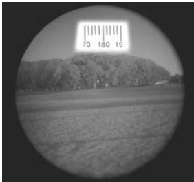
FIGURE 2-13. VIEW THROUGH INSTALLED COMPASS
