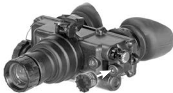
FIGURE 2-5. INSTALLATION OF THE IR SPOT/FLOOD LENS
